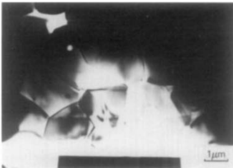
FIG. 5. Transmission electron micrograph showing garnet microstructure in YAS-4.
